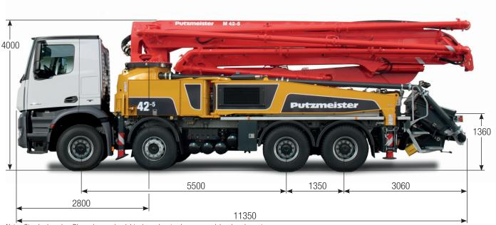
Note: Standard version. Dimensions and weights depend on truck, pump model and equipment. Dimensions in mm, MB-Actros 3241, Euro 5 as example.
